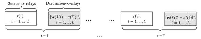
Fig. 4:  $T$  rounds of time slots for the forward (source-to-relay) and backward (destination-to-relay) pilot sequences.
